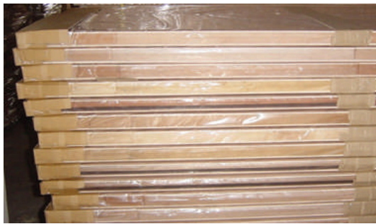
Figure 5.1 Door panels protected with polythene sheets
