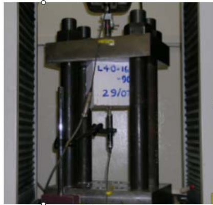
Study on bond strength & Bond stress vs slip behavior of various HSLWCs
