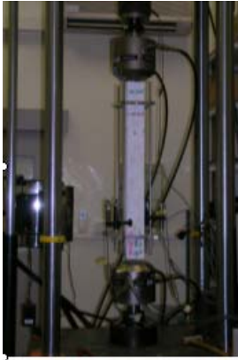
Study on bond strength & Bond stress vs slip behavior of various HSLWCs
