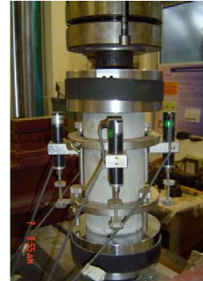
Study on modulus of elasticity and stress-strain behaviour
