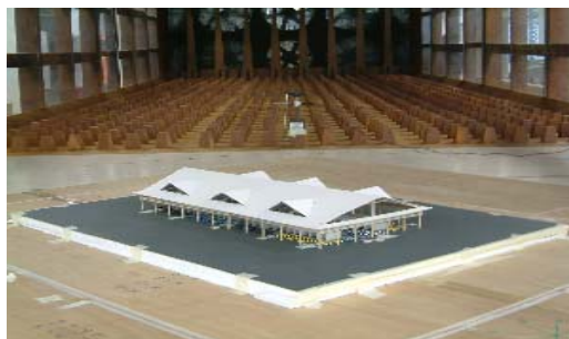
Figure 1. Wind tunnel and scaled model
