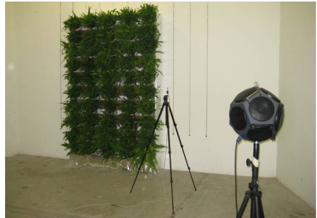
Fig 4: Acoustics experiment setup of vertical greenery system inside reverberation chamber
