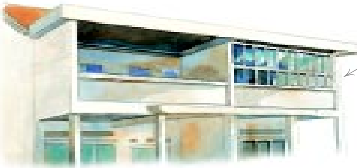
Enclosing of balcony with glass panels
