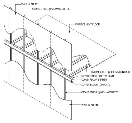
Figure 9.12 Steel frame wall & flooring using C-sections
