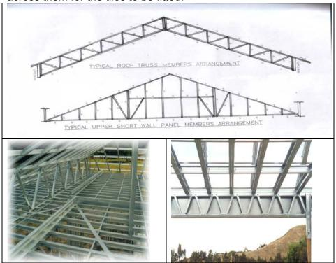
Figure 9.17 Roof Truss
