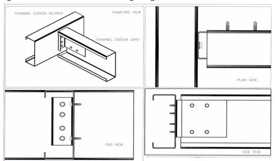
Figure 9.13 Joist to C-Section Bearer Connection for Flooring Details recommended by BHP Steel Lysaght
