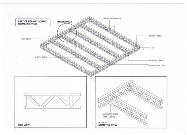
Figure 9.14 Lattice Beam Flooring
