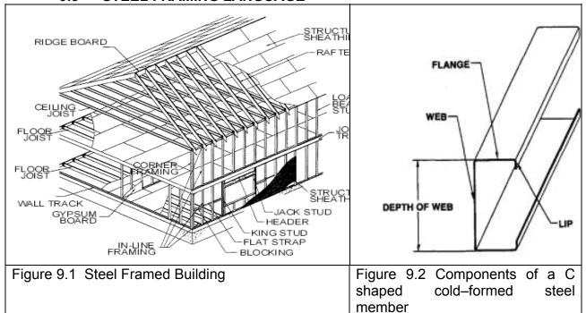
**Bottom Plate:** A plate that contains the bottom end of a wall stud. The top plate has a web and flanges, but no lips.
