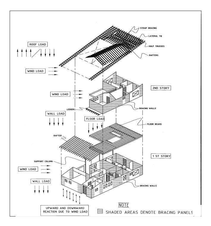
Figure 9.3 Loading Path Diagram
