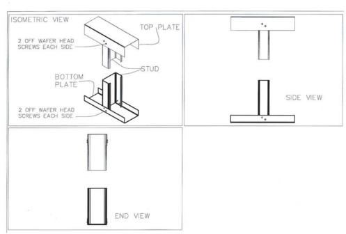
Figure 9.6 Stud to Plate Connection
