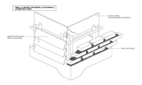
Figure 9.11 Internal & External Wall cladding
