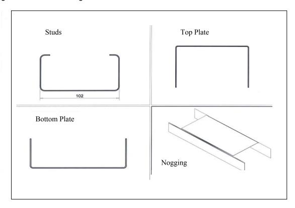
Figure 9.5 Studs, Plates & Nogging Sections Details recommended by BHP Steel Lysaght
