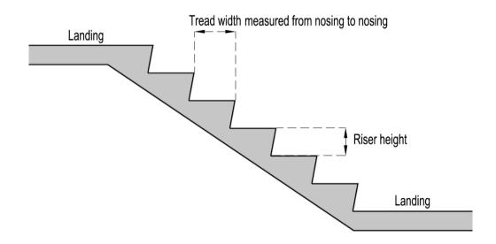
Figure E.3.4.2(a) - Measurement of Tread and Riser
