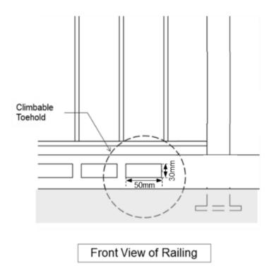
Figure H.3.4A.1(c) - Toehold Dimensions at Railing
