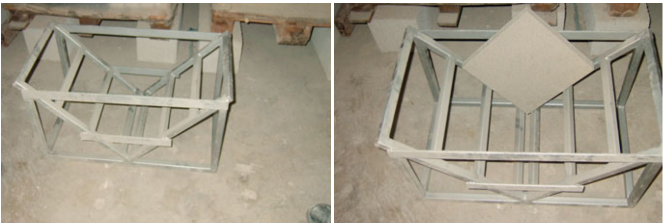
Fig. 3.6 – Gauge box used on site to group tiles according to size.
