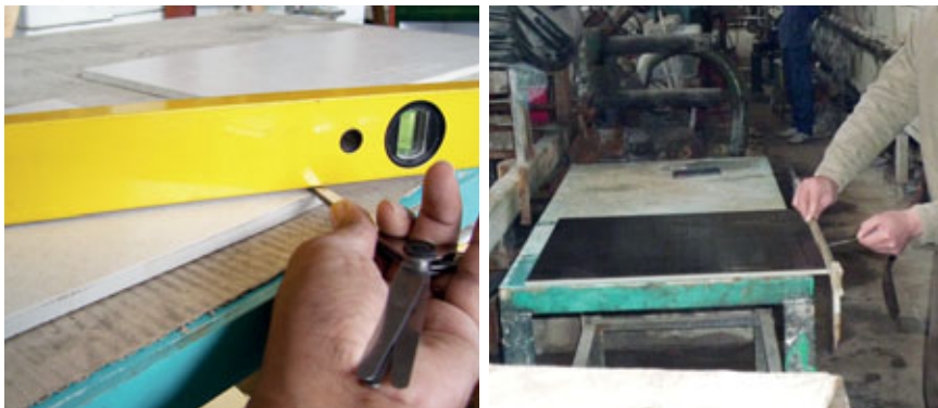
Fig. 3.8 – Warpage on tiles may occur after the firing and cooling process.
