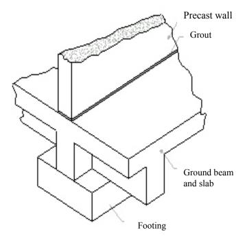
Figure 3.5 Footing below precast load bearing walls
