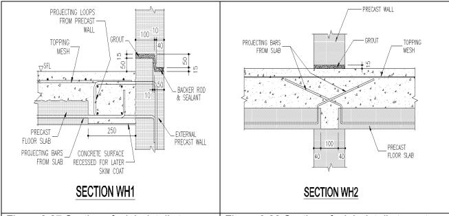
Figure 3.27 Section of slab details to facade walls
