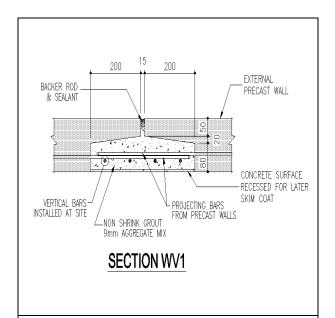
Figure 3.16 Plan of connection for long panel of facade walls or end walls
