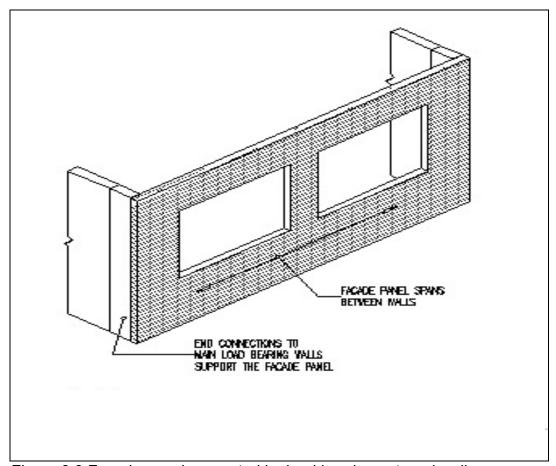
Figure 3.9 Facade panel supported by load bearing external walls
