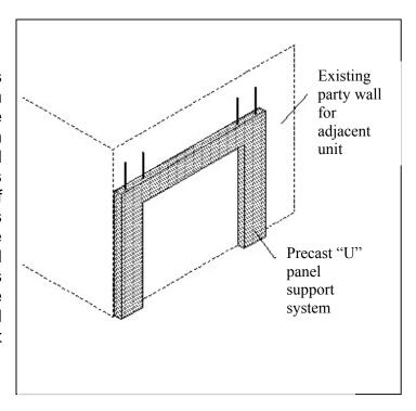
Figure 3.8 Precast load bearing wall for infill unit
