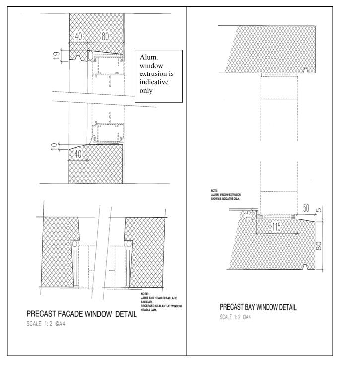
Figure 3.11 Opening for Window at precast facade wall
