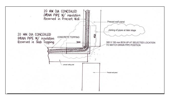
Figure 3.30 Option 1 - Proper co-ordination at interface between horizontal vertical element
