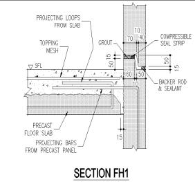
Figure 3.17 Section of water-stop detailing for wall-slab system
