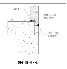
Figure 3.18 Section of water-stop detailing for beam-slab system
