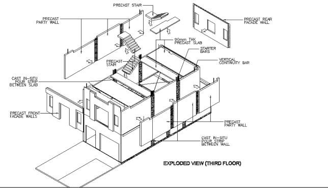
Figure 3.3 Precast prestressed slabs spanning between walls with composite in-situ topping for 3<sup>rd</sup> storey
