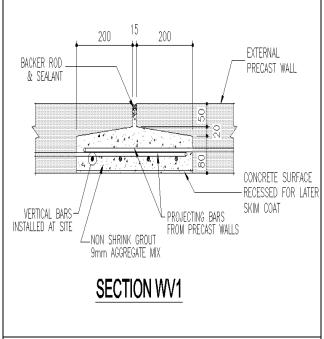
Figure 3.29 Section of slab details to pour strip of party walls
