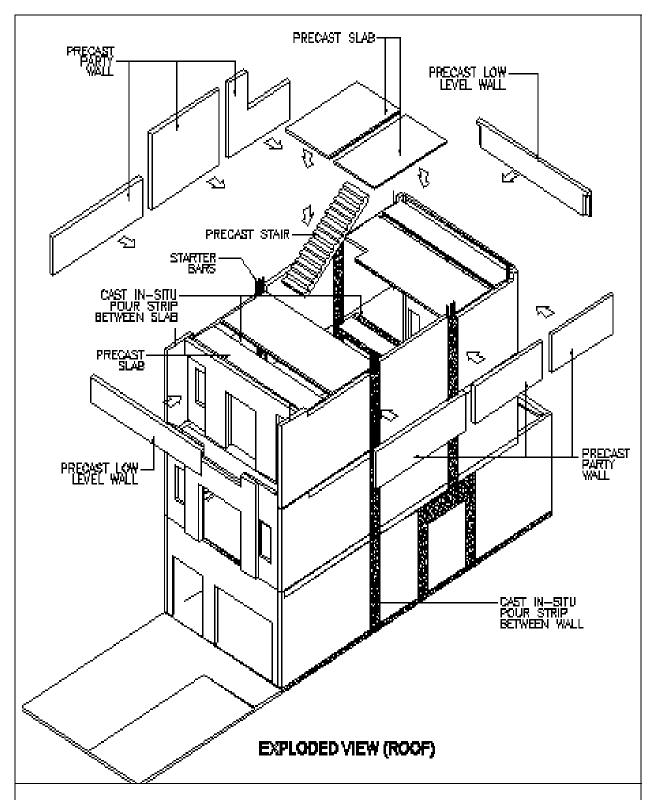
Figure 3.4 Precast prestressed slabs spanning between walls with composite in-situ topping for roof
