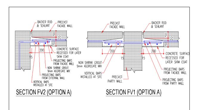
Figure 3.19 Option A - Plan of connection between end wall and facade wall
