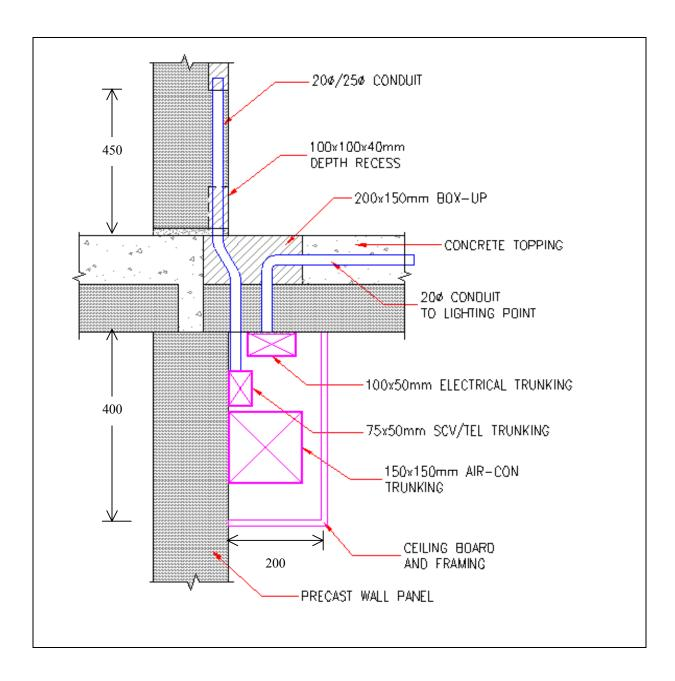
Figure 3.32 Option 2 - Using external tray
