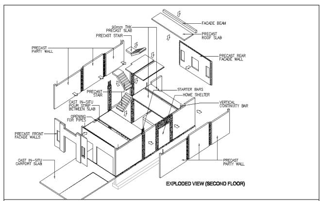
Figure 3.2 Precast prestressed slabs spanning between walls with composite in-situ topping for 2<sup>nd</sup> storey
